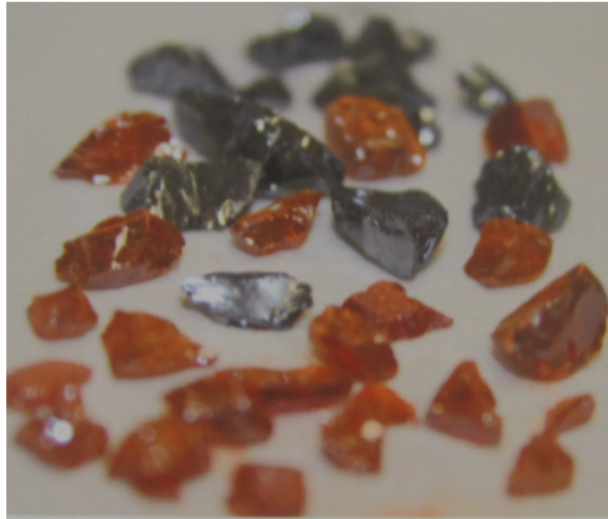
Figure 3.5: Pieces of chalcogenide glasses. Orange= \text{As}_2\text{S}_3 (Arsenic sulfide) Black= \text{As}_2\text{Se}_3 (Arsenic selenide).
